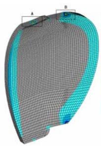
Nonlinear analysis result (thickness = 0.75 mm, blood pressure = 400 KPa)
