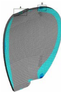
Linear analysis result (thickness = 0.5 mm, blood pressure = 40 KPa)
